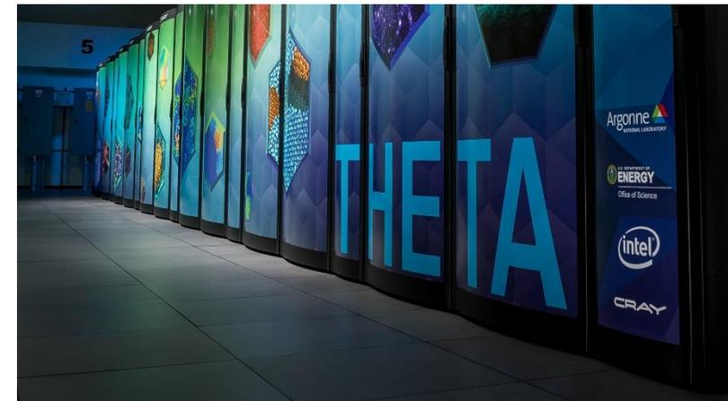
Argonne Theta Supercomputer (4096 Intel Xeon Phi cards)
